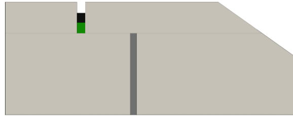
Joints of exposed 6mm Everest Heavy Duty Fiber Cement Board sealed with primer modified mortar
