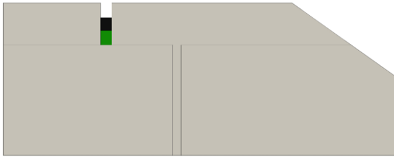
Joints of Internal 9mm Everest Heavy Duty Fiber Cement Board sealed with backer rod & sealant
