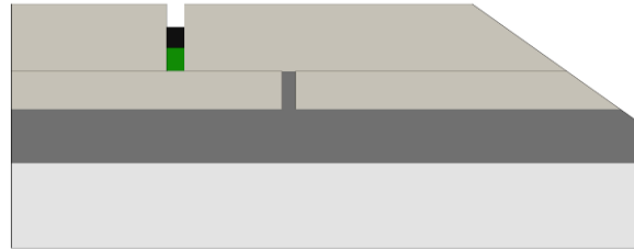
Pasting of EPS over modified mortar
