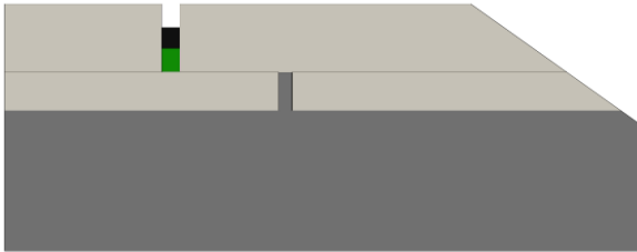
Application of base coat modified mortar
