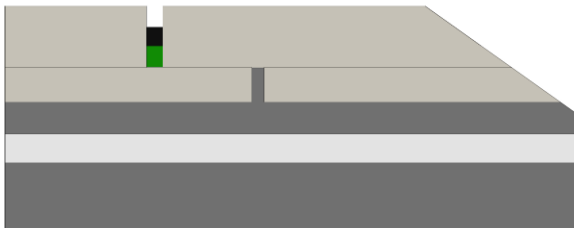
Application of second coat modified mortar base coat over EPS
