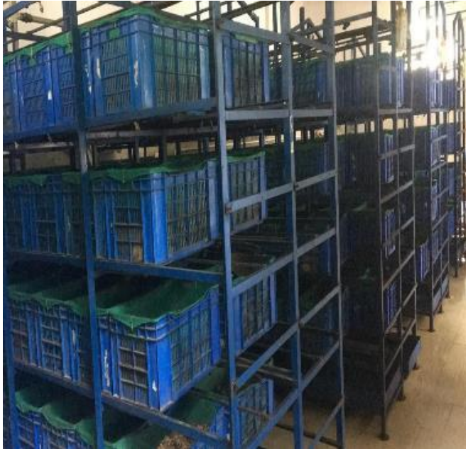
Composting in Crate system for converting decompose food waste into organic manure
