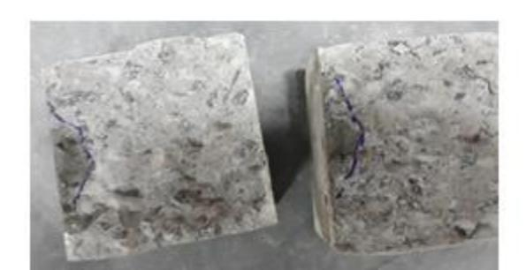
Concrete Sample after VVater Permeability Test
