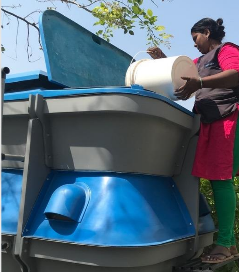
Segregated wet waste is added into composters
